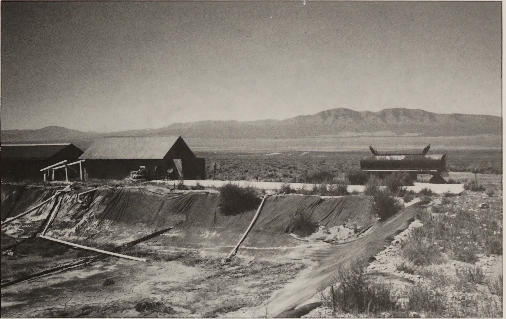
Figure 2. Numerous rips in the liner are visible.
